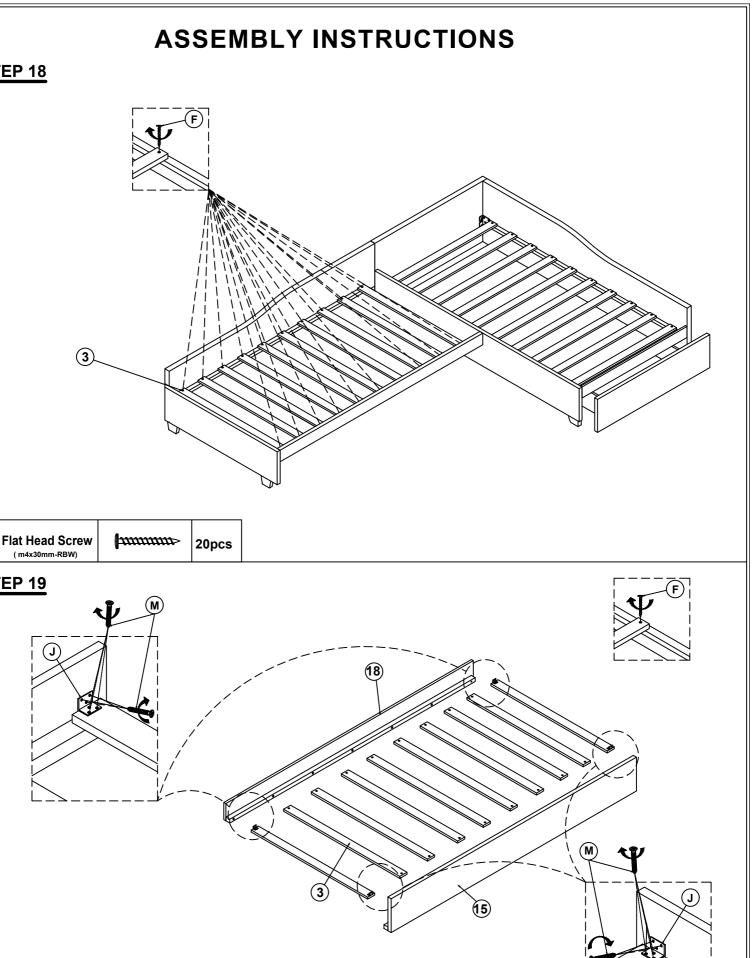
**Flat Head Screw** www. 24pcs ( m4x15mm-RBW) |mmmm> **Flat Head Screw** 20pcs ( m4x30mm-RBW) **Square Patch** 4pcs 38mmx38mmx25mmx2mm MADE IN VIETNAM
